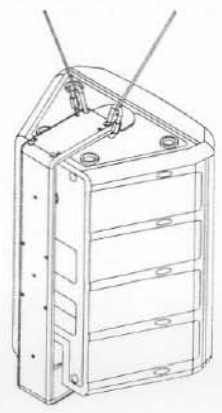
Figure 7—Sx100 Suspending the Sx100 Using Mb200 Installation Kit
